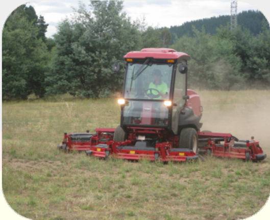
Another significant investment was the Toro Ground Master Wide Mower which cuts up to 3 times faster and has better fuel economy than the mower it replaced. It complies with US Tier 3 emissions standards for non diesel engines and can also run on biodiesel. Photo courtesy of Alpine Shire Council.
